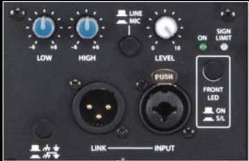
Selectable MIC/LINE input with 2-band EQ
