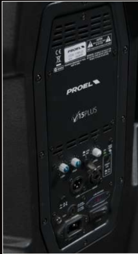
Ultra-lightweight, high-efficiency Class D power amplifiers with SMPS
