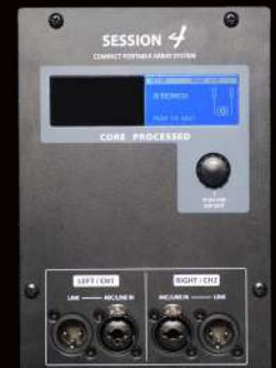
User-friendly control interface with single knob and large LCD
