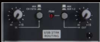
USB interface with routing options for PC recording and playback
