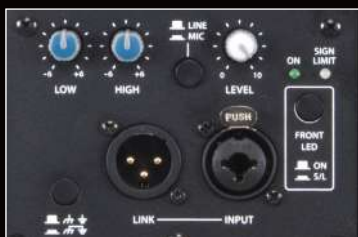
Selectable MIC/LINE input with 2-band EQ
