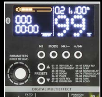
24bit studio-grade digital effect with 99 presets with adjustable parameters and LCD color display
